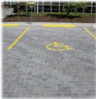
**A:** Yes. ADA Design Guidelines require that surfaces be firm, stable and slip resistant. PICP designs can provide a firm and stable surface for visually impaired persons and those using wheeled mobility devices. If the openings in the surface are not desirable, solid units can be used in areas subject to disabled persons. Such areas might include designated spaces in parking lots.
