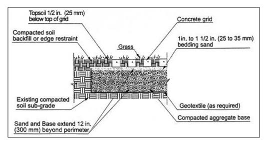
Filter cloth is recommended for use with low CBR soils (less than 4%), those with high clay and silt contents, soils in high water table areas, or soils in low lying areas subject to flooding. The filter cloth is placed over the compacted subgrade. The filter cloth should be fine enough to prevent migration of soil into the gravel base. Woven fabrics are preferred over non-woven materials when the cloth is placed directly under the sand layer in installations subject to traffic.
